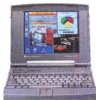
TravelMate 4000M/50 i486SX2/50 MHz HD 340 / 200 MB Display Colore TFT / DS
